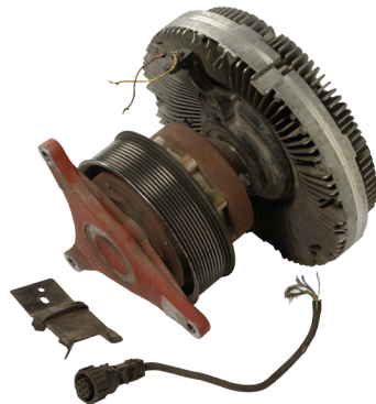
Fan drive damage caused by a frayed or broken belt
